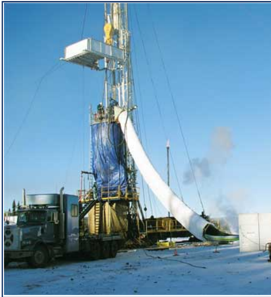
Fig. 1 . The tube-like controlled-descent escape method (here by FoxxHole) meets IRP15 requirements. The "pole slide" will be disallowed in January 2009 in British Columbia.
